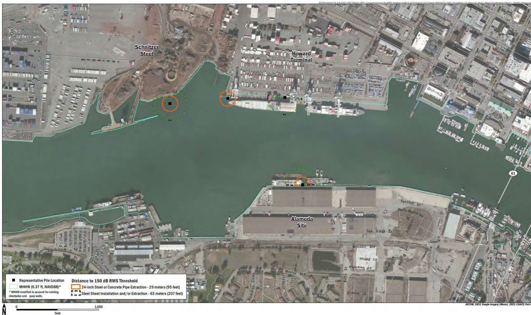
Figure 6-1 Estimated Distance to In-Water Sound Pressure Criteria for Fish for Vibratory Driving
